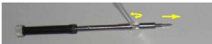
FIG 1-24 REMOVING KNIFE FROM THE TANGENTIAL KNIFE HOLDER
