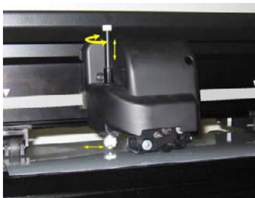
FIG 1-26 INSERTING THE TANGENTIAL KNIFE HOLDER
