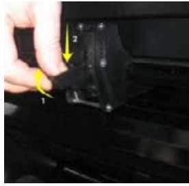
FIG 5-1 LIFTING THE PINCH ROLLER
