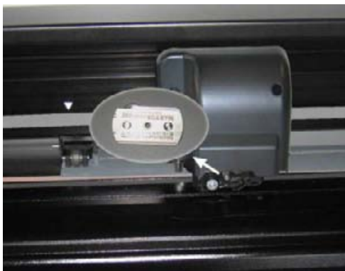
FIG 1-35 RAZOR BLADE FOR AUTOMATIC SEPARATION OF MEDIA
