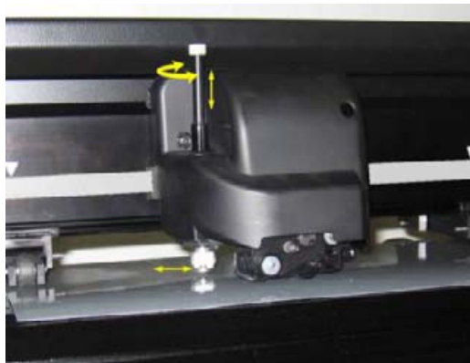
FIG 1-23 REMOVING THE TANGENTIAL KNIFE HOLDER
