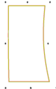
Example of a distorted outcome with its printed and cut lines (overlap entirely)
