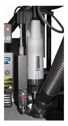
The router module has a motor capable of handling most used solid boards in the graphic and sign industry.
