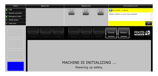
Click to proceed with the startup sequence. In the next step the emergency buttons will be checked and after that the safety trip switches and the safety light beams.
