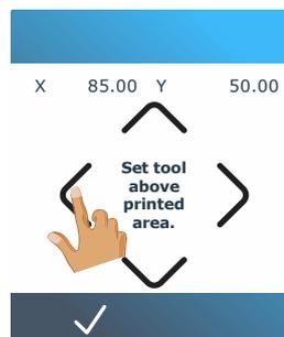
8. Use the arrows to manoeuvre the knife in a printed area.
