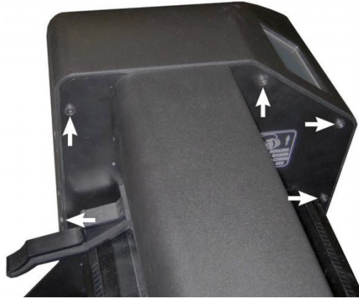
FIGURE 1 REMOVING RIGHT HAND COVER.
