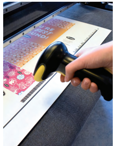
Barcode Workflow with hand scanner
