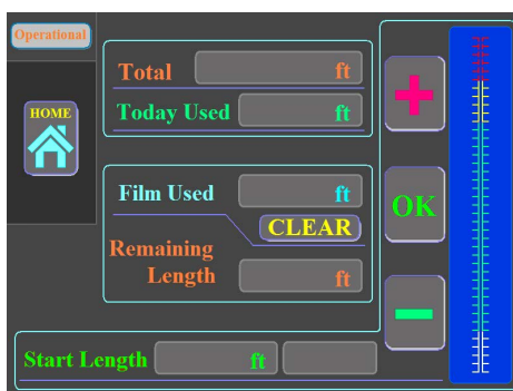
FILM USAGE COUNTER Tracks the film usage per job, per day, and lifetime.
