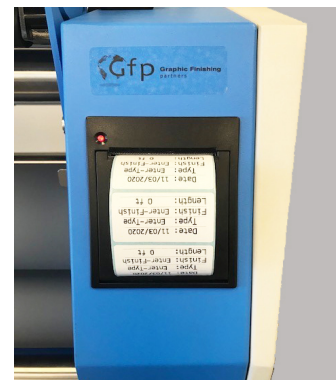
ROLL LABEL PRINTER generates pressure sensitive label with film description and remaining footage for labeling partial film rolls.
