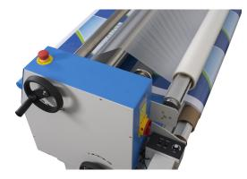
Motorized rear rewind for roll-to-roll applications
