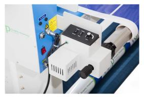
Motorized rear rewind for roll-to-roll applications
